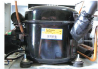
Reciprocating Hermetic Seal type Compressor
